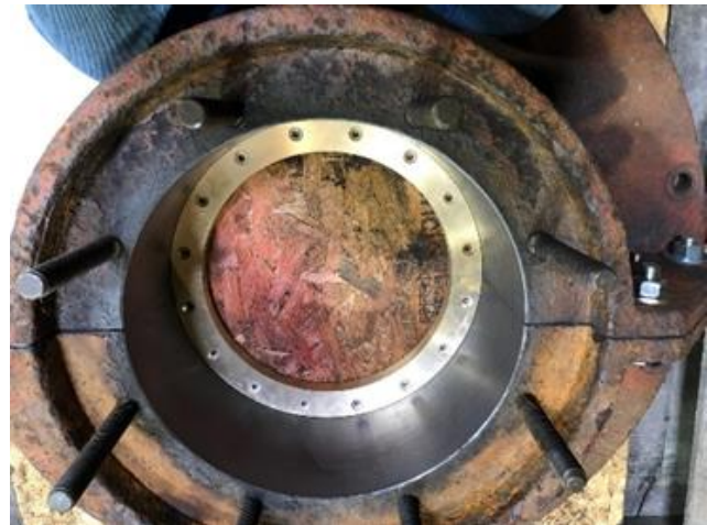
Figure 2 Refurbished Packing Box
