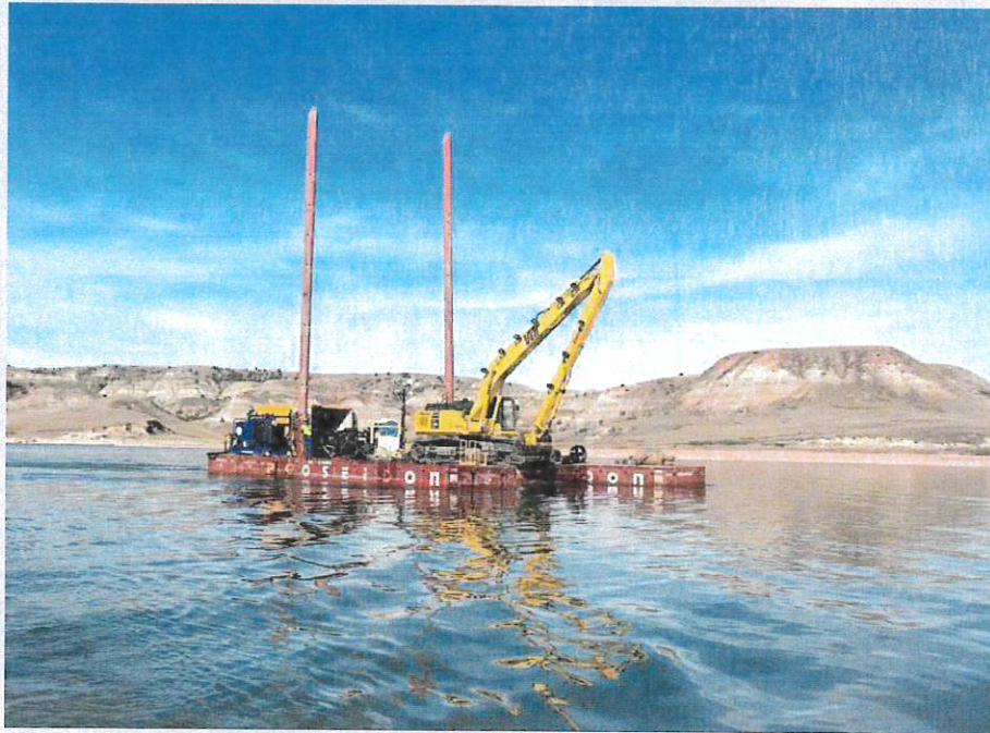
Figure 1 depicts a fully assembled flexifloat pontoon system.
